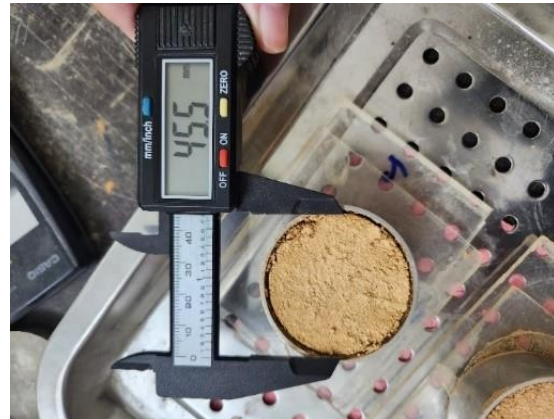
Figure 5. Measuring the diameter of the SC specimen
