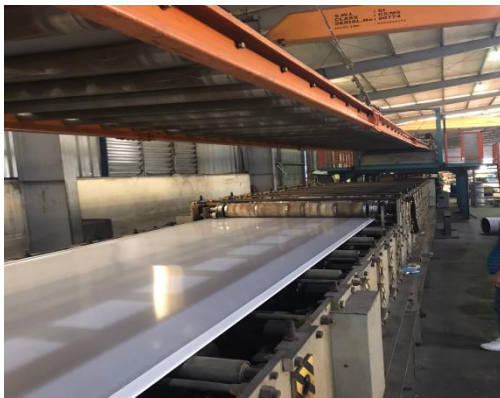
Pressing the top of corrugated iron
