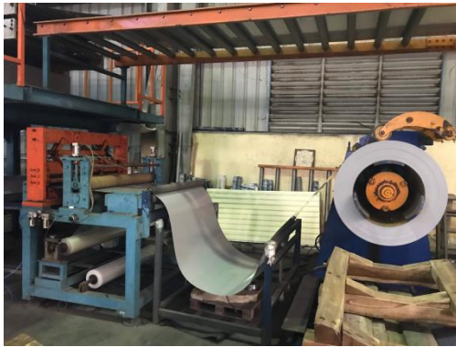
Flattening corrugated iron
