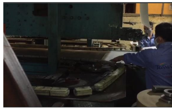
Positioning the corrugated iron into the PU injection mold
