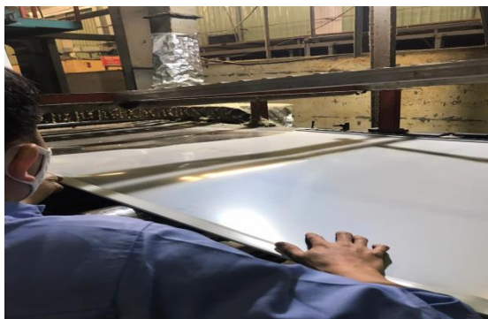
Putting corrugated iron into the fixture
