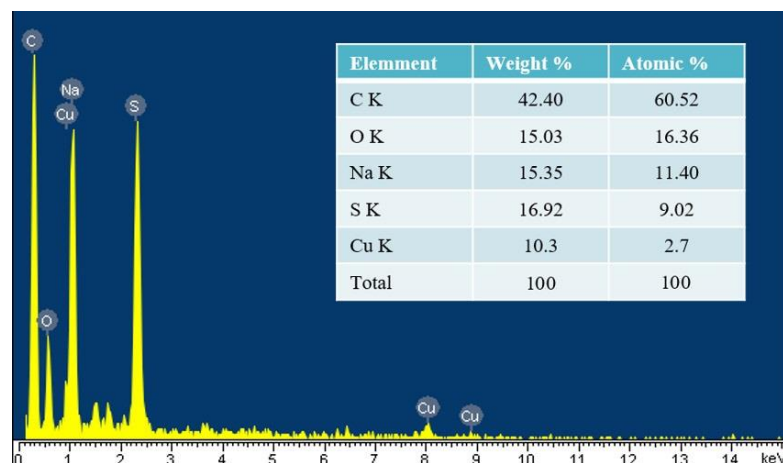
Figure 5. EDS analysis of rGO-CuS SC electrode.
