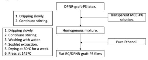
Figure 2. Scheme of blending RC with DPNR-graft-PS.
