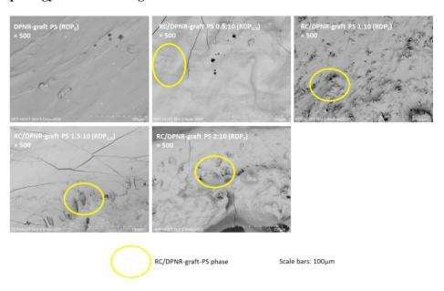
Figure 6. SEM images of analyzed samples with different RC: DPNR-graft-PS ratios.
