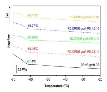
Figure 9. DSC curves of DPNR-graft-PS and RC/DPNR-graft-PS.
