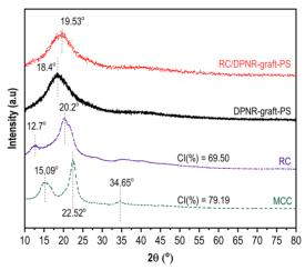
Figure 5. XRD of MCC, RC, DPNR-graft-PS and RC/DPNR-graft-PS.
