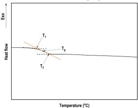
Figure 3. Method for determining T<sub>g</sub> via DSC.
