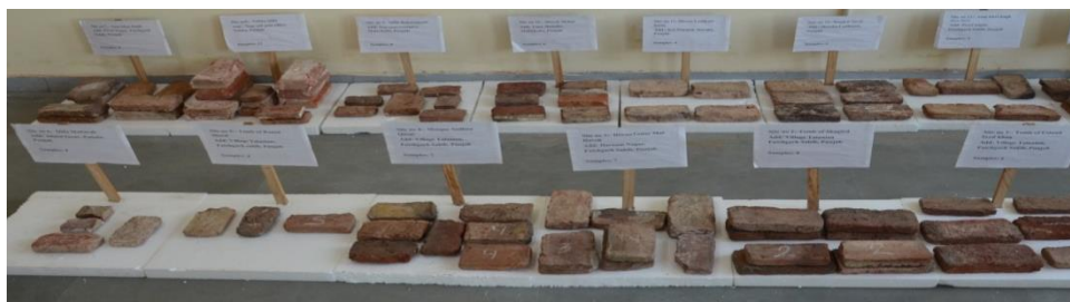
Figure 3. Collected heritage Nanakshahi clay bricks (NSCB) from selected sites (thickness: 3 - 3.9 cm).
