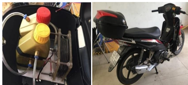
Figure 4. Installation of Dry-Type HHO Gas Generator into motorcycle.
