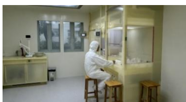
Figure 1. The ISO 5 class, metal-free chemical clean room at the Institute of Geological Sciences, Vietnam Academy of Science and Technology (VAST).
